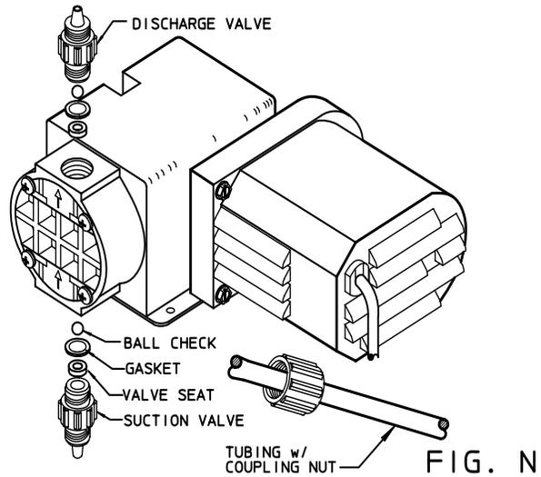
5. Be sure the drive bracket assembly is in the **fully retracted position** when installing the new diaphragm. Install the new diaphragm by screwing it in hand tight, then, back off one-fourth turn or until screw holes are lined up.
